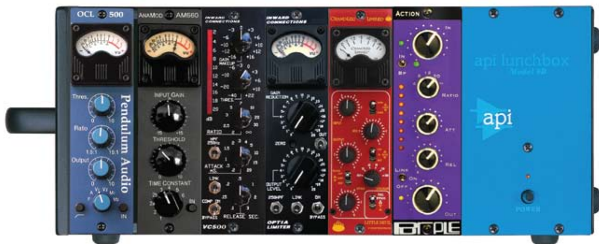
API's six-slot Lunchbox housing sparked a movement toward using 500 Series format modules as outboard processors. Shown here are the six modules tested this month: (left to right) Pendulum Audio OCL-500, AnaMod AM660, Inward Connections VC500 and OPT1A, Chandler Limited Little Devil, and Purple Audio Action.
