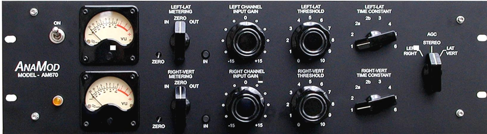
**Input Gain** The INPUT controls are continuously adjustable from -15dB to +15dB. Unity gain is at the center position.
